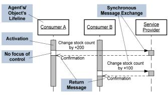
**Relation to other diagram types:** The connection of the agents via channels is shown in Component / Block diagrams. To show more details of processing, use Activity diagrams.
