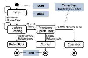
A state transition is performed when the event occurs (given the guard condition is met). The transition may include an action that has to be executed as well.
