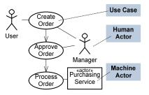
**Relation to other diagram types:** Use Component / Block diagrams to show which agents will perform which tasks. Use Activity, Sequence or State Machine diagrams to display the behavior described by the tasks.
